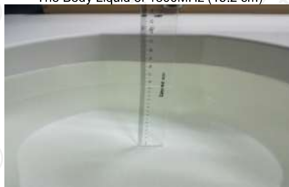
The Body Liquid of 2450MHz (15.3cm)
