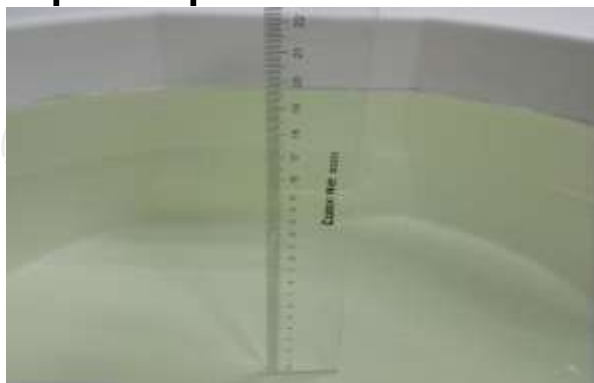
The Body Liquid of 835MHz (15.4cm)
