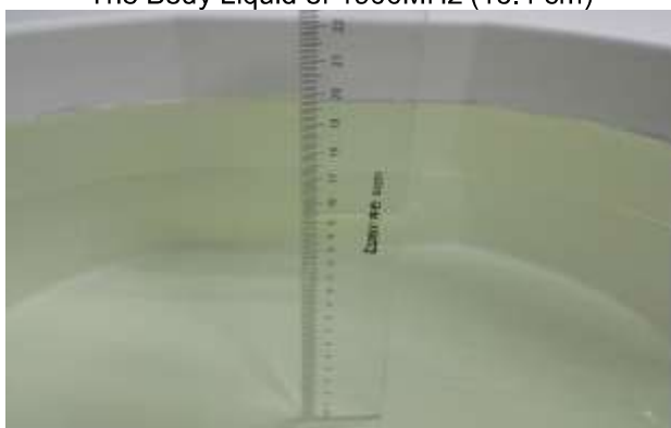
The Body Liquid of 750MHz (15.4cm)
