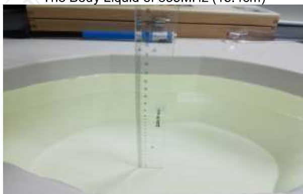
The Body Liquid of 1900MHz (16.4 cm)
