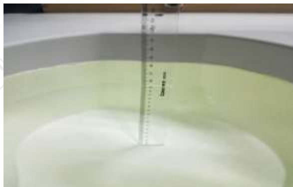
The Body Liquid of 1800MHz (15.2 cm)
