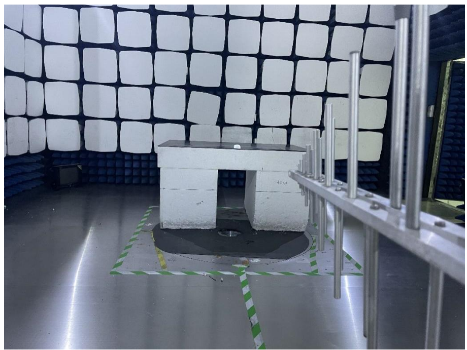
Radiation Emission Test Setup (30MHz to 1GHz)
