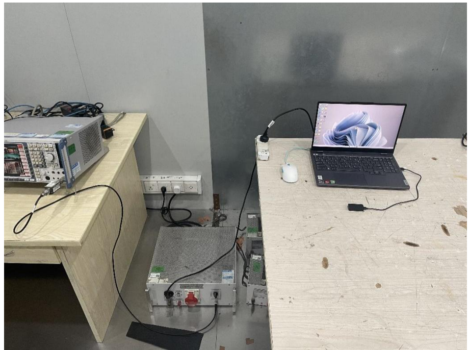
Conducted Emission Test Setup
