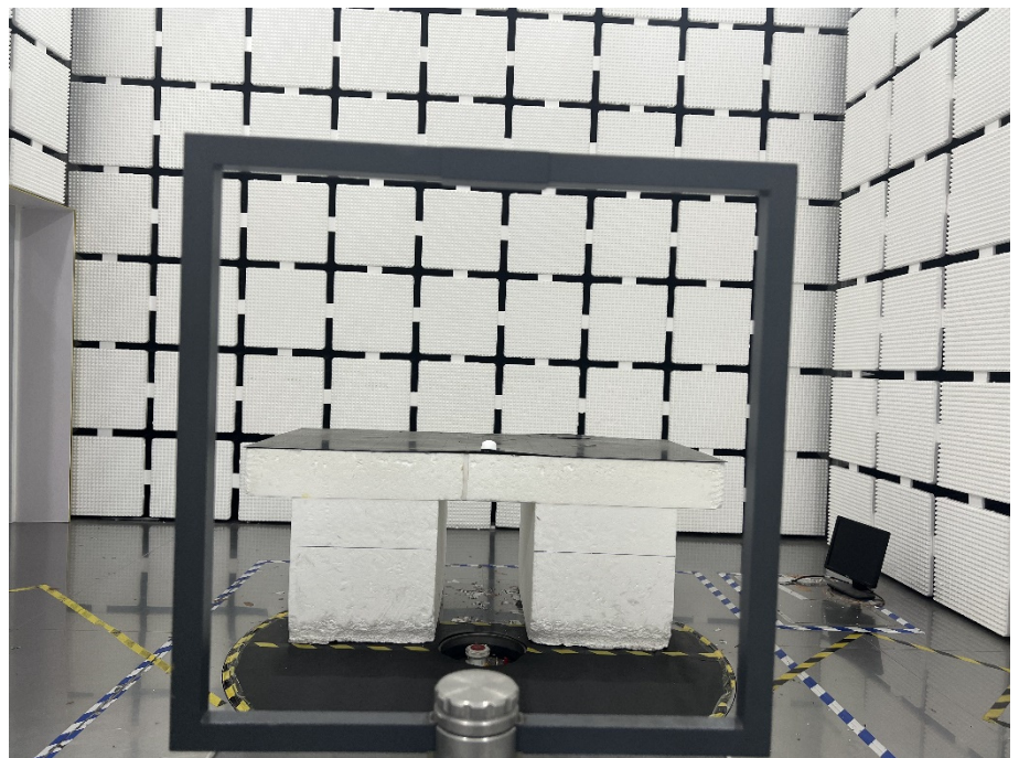
Radiation Emission Test Setup (Below 30MHz)
