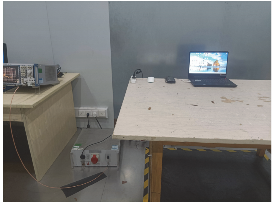
Conducted Emission Test Setup
