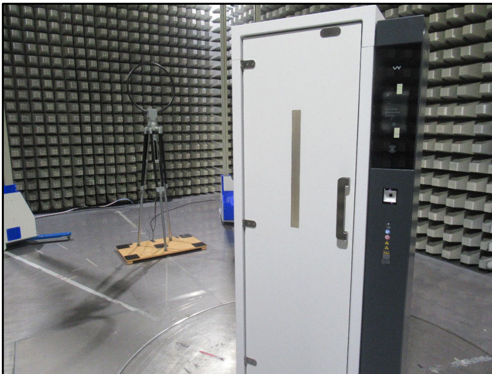
Photo 2 Radiated Test Setup-9 kHz – 30 MHz
