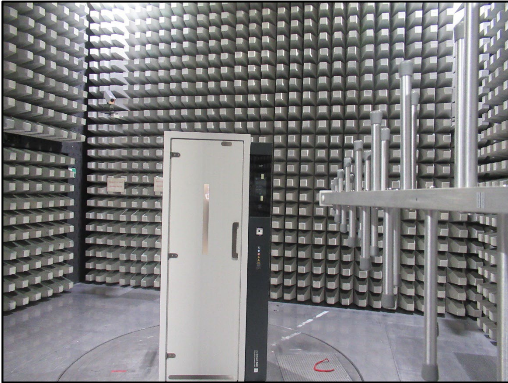
Photo 3 Radiated Test Setup-30 MHz – 1 GHz
