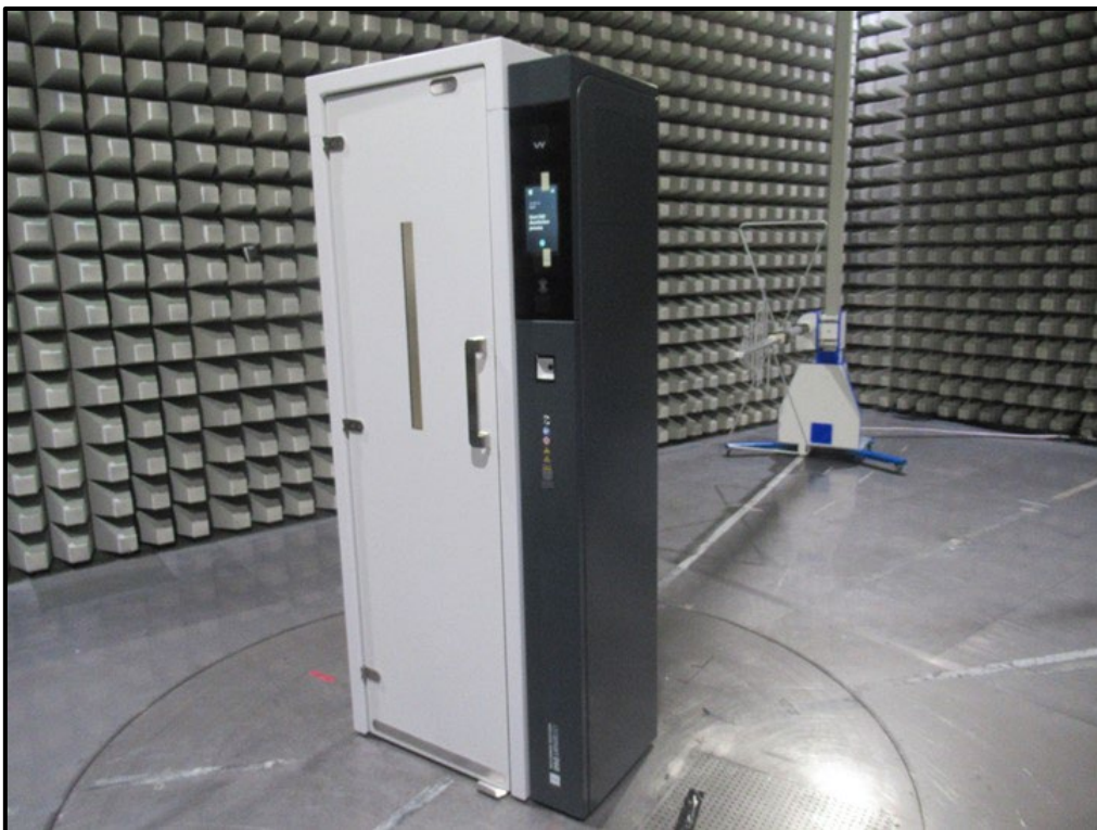
Photo 4 Radiated Test Setup-30 MHz – 1 GHz
