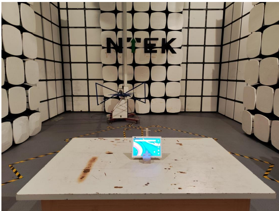
Radiated Measurement Photos(30MHz~1GHz )
