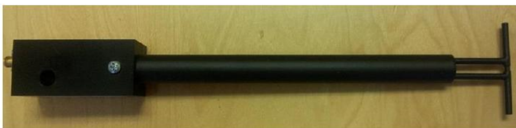
Figure 1 – MVG COMOSAR Validation Dipole
