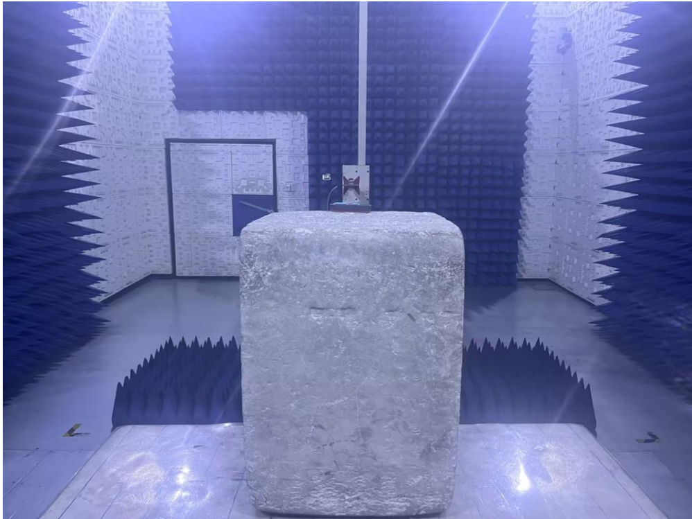
RADIATED EMISSION TEST SETUP ABOVE 1GHz
