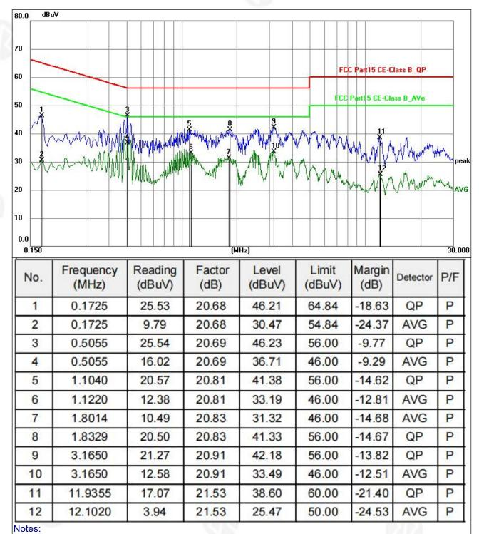
1.An initial pre-scan was performed on the line and neutral lines with peak detector.
