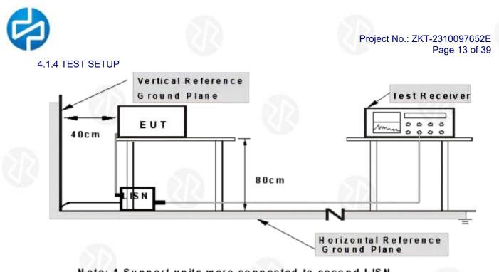
Note: 1.Support units were connected to second LISN. 2.Both of LISNs (AMN) are 80 cm from EUT and at least 80 from other units and other metal planes
