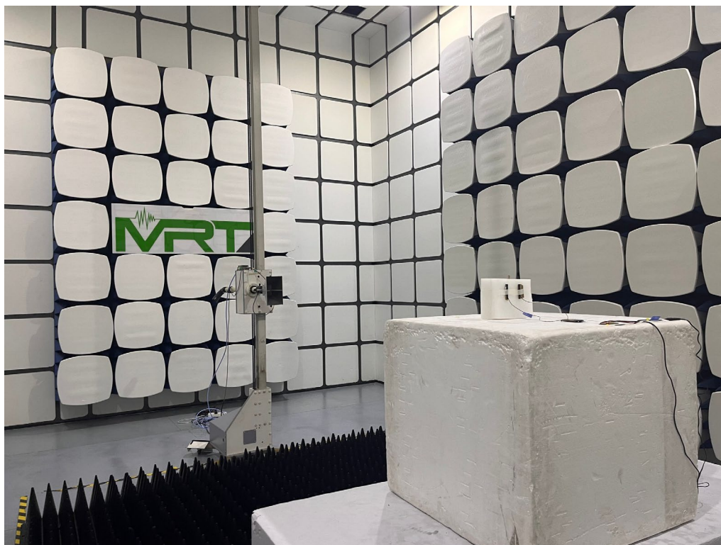
Description: Radiated Restricted Band Edge Test Setup for Ant 1
