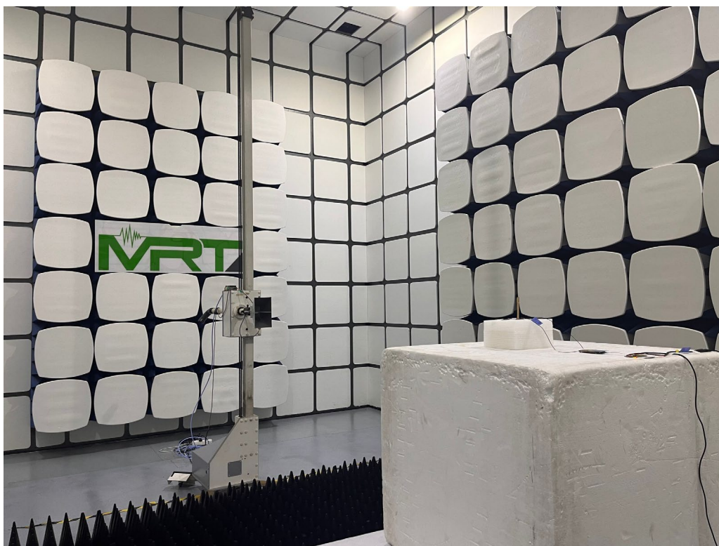
Description: Radiated Spurious Emission Test Setup for Ant 1 Above 1GHz
