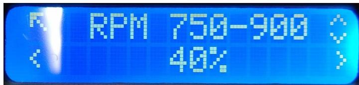
Advanced menu to control how quickly the gun will limit the recoil to avoid overheat (such as if you made all weapons have 100% recoil power, this will clamp the motor after X bullets to cool it down for Y seconds). Suggested to leave all these menus at defaults.
