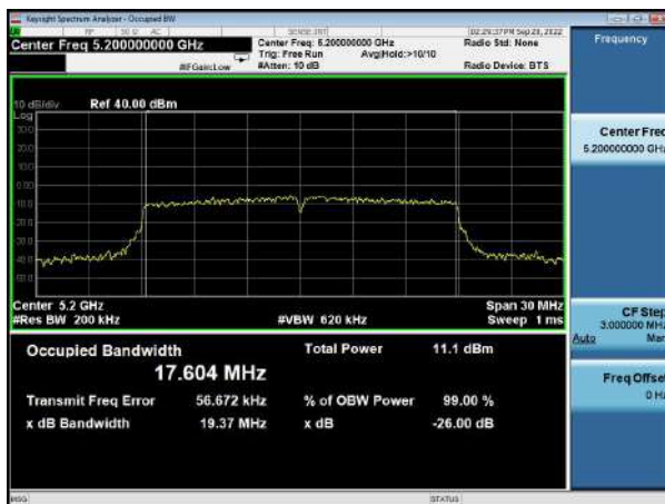
(802.11ac20) 26dB Bandwidth plot on channel 40
