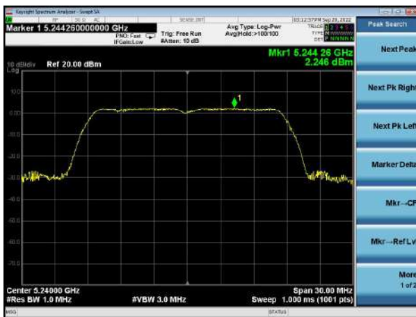
(802.11ax20) PSD plot on channel 48
