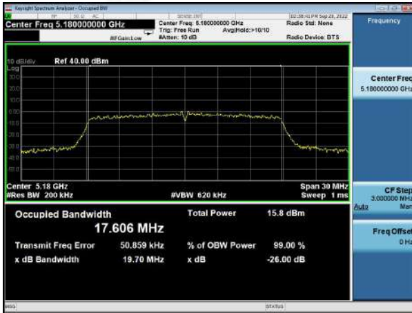
(802.11ax20) 26dB Bandwidth plot on channel 40
