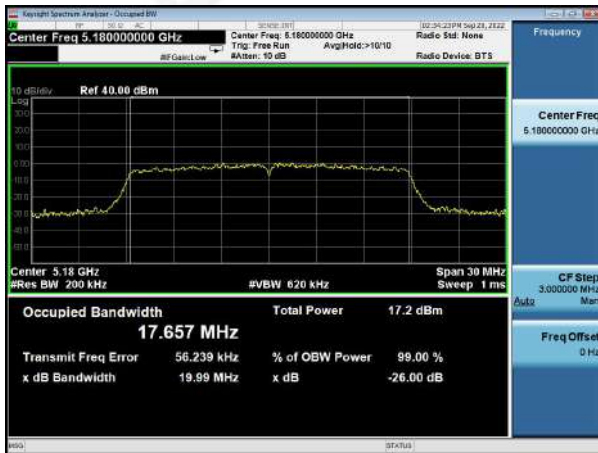
(802.11 n20) 26dB Bandwidth plot on channel 40
