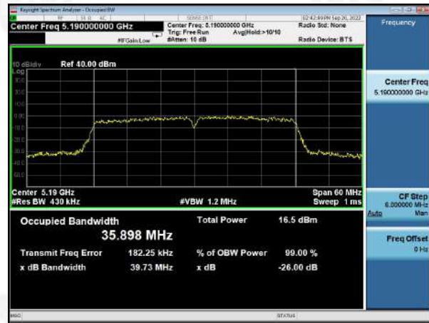
(802.11 n40) 26dB Bandwidth plot on channel 46
