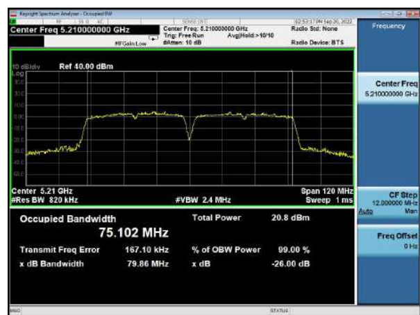
(802.11ac80) 26dB Bandwidth plot on channel 42
