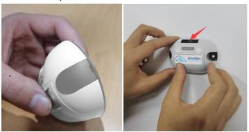
2-4-5. Fix the right screw first but not locked, then the left. Adjust the position of the horizontal bubble again, and then lock the screw. (there is a punching position drawing at the end of the manual)
