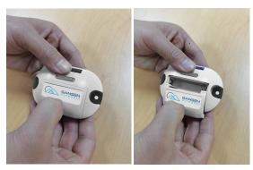
1-1-4.Install 2 AAA batteries and close the battery cover (Note: it is recommended to turn off the device switch if it is not used for 3-6 months. It is recommended to take out the batteries if it is not used for more than 6 months to avoid any corrosion)
