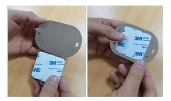
2-3-3. First adjust the the RV level, put the upper edge of the Device close to the position to be installed (the installation direction can only be parallel or perpendicular to the driving direction of the vehicle, not inclined installation). *Keep the bubble facing up and in the middle*. The device shall be installed vertically and horizontally.
