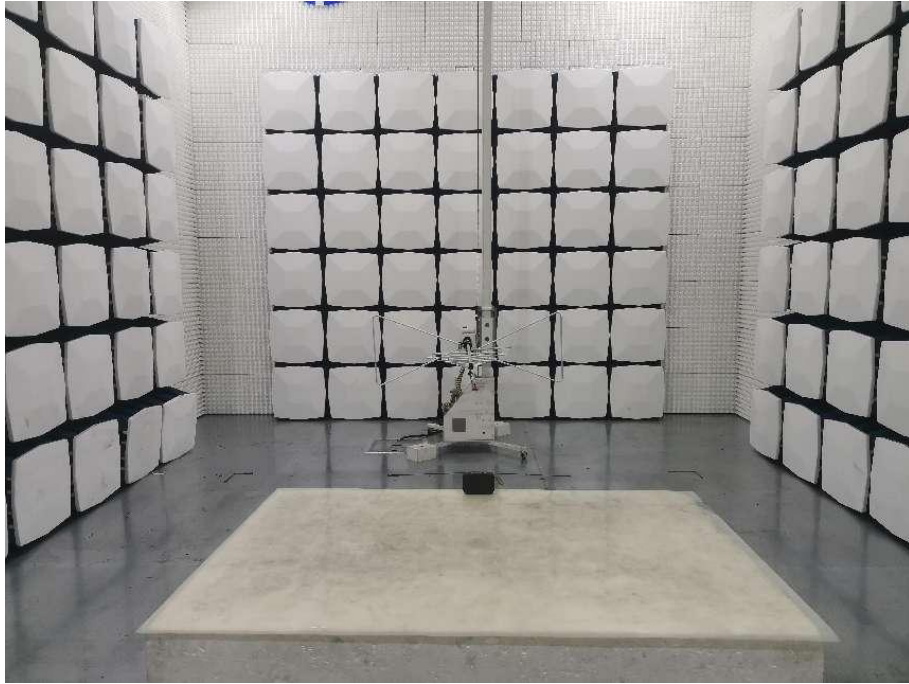
RADIATED EMISSION MEASUREMENT (below 1G)
