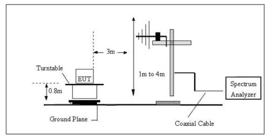
(C) Radiated Emission Test-Up Frequency Above 1GHz
