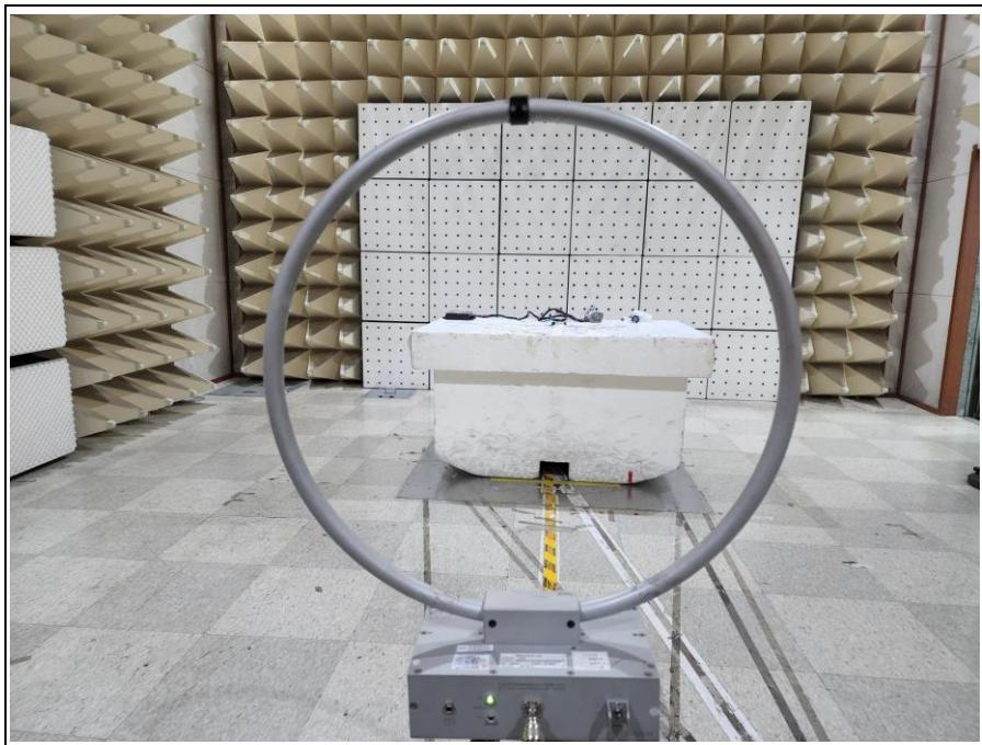
**3. Photo of Radiated Spurious Emission Test (30 MHz ~ 1 000 MHz)**
