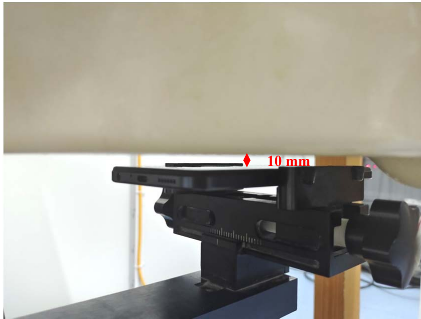
Body (Worn) Front Setup Photo (10mm)
