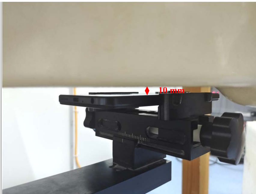
Body (Worn) Back Setup Photo (10mm)
