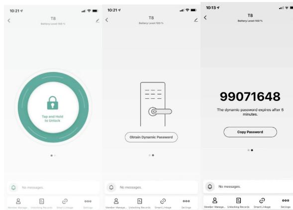
Swipe left on interface 1; enter interface 2; click "Get dynamic password" on interface 2; generate a dynamic password; enter the password at the fingerprint password lock end to unlock.
