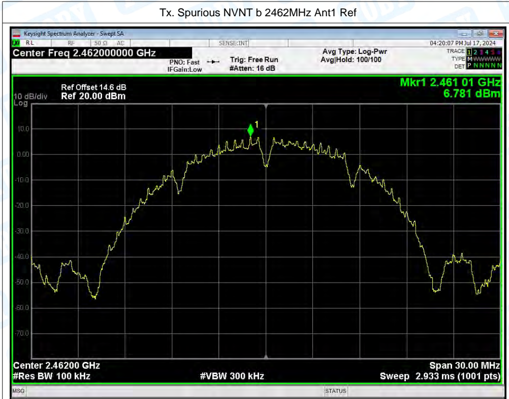
Tx. Spurious NVNT b 2462MHz Ant1 Emission
