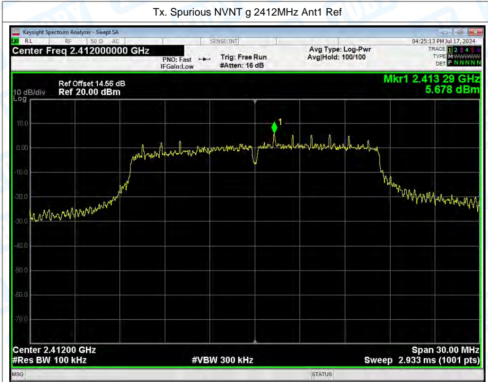
Tx. Spurious NVNT g 2412MHz Ant1 Emission
