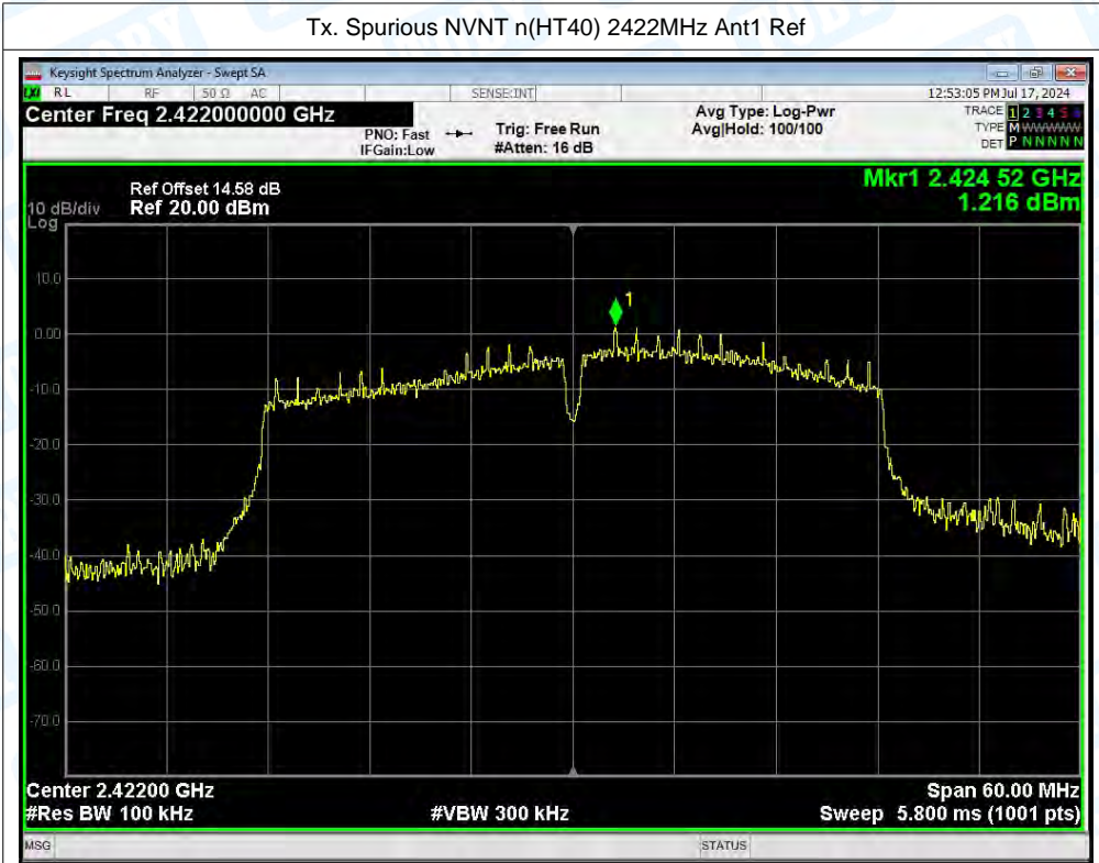
Tx. Spurious NVNT n(HT40) 2422MHz Ant1 Emission
