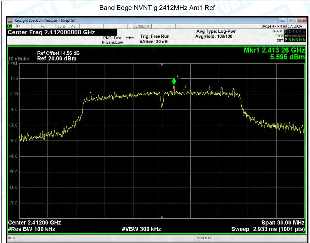
Band Edge NVNT g 2412MHz Ant1 Emission
