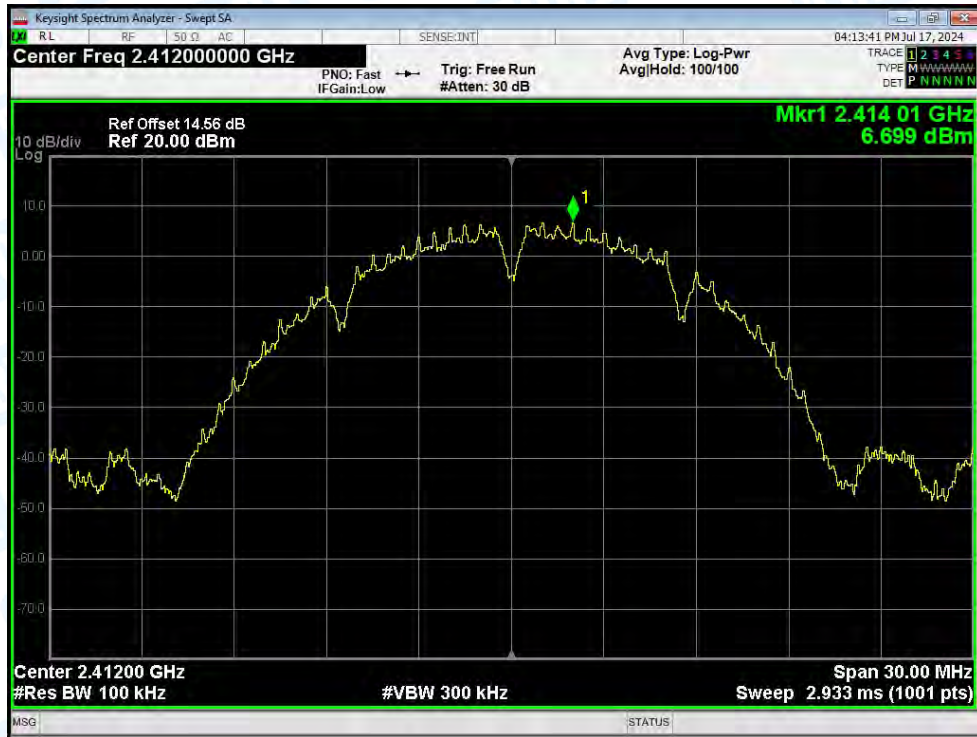
Band Edge NVNT b 2412MHz Ant1 Emission
