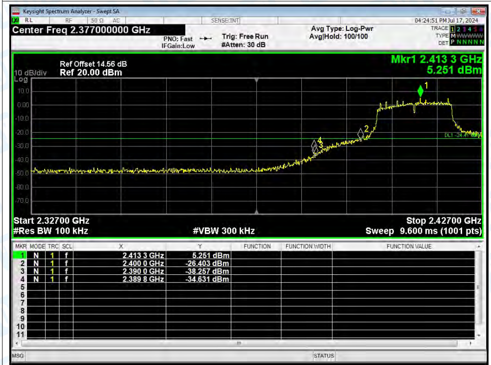
Band Edge NVNT g 2412MHz Ant1 Emission
