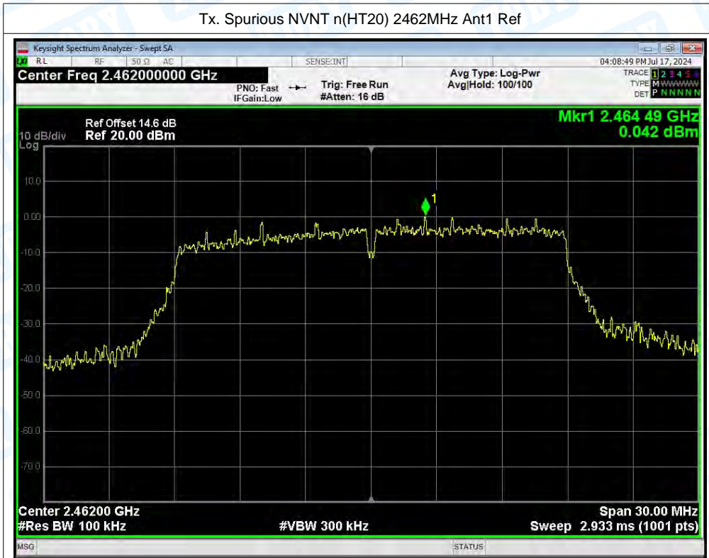
Tx. Spurious NVNT n(HT20) 2462MHz Ant1 Emission
