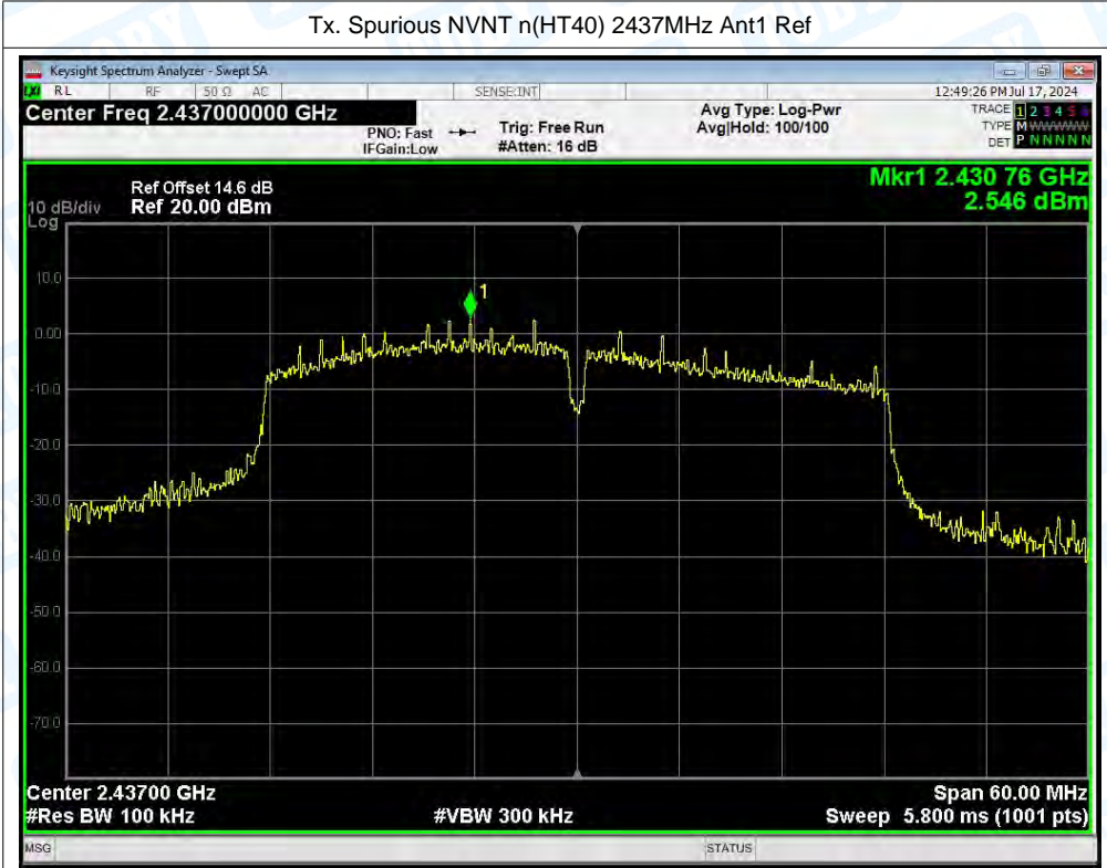
Tx. Spurious NVNT n(HT40) 2437MHz Ant1 Emission
