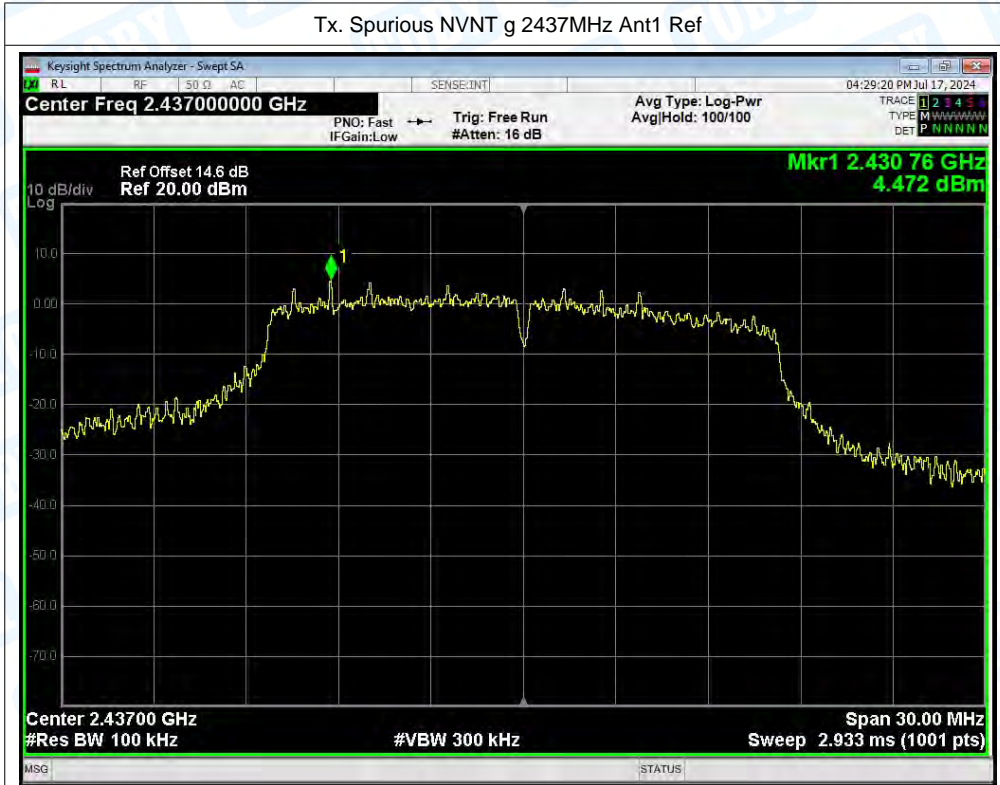
Tx. Spurious NVNT g 2437MHz Ant1 Emission
