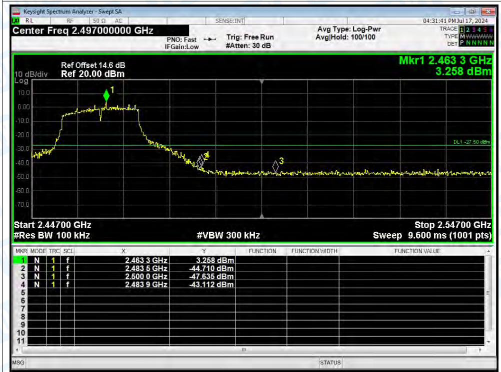
Band Edge NVNT g 2462MHz Ant1 Emission
