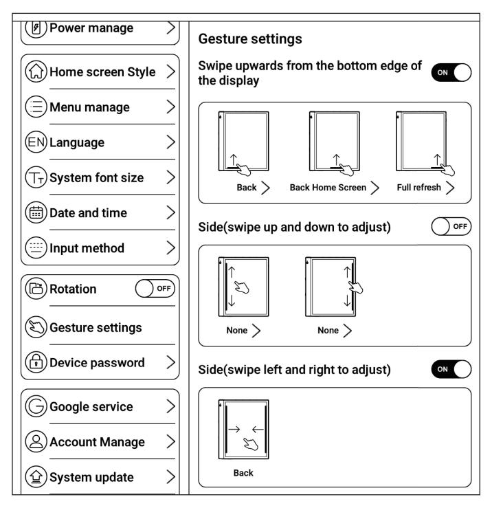
By default, upward swipes from the bottom and left-right swipes from the sides are enabled, while up-down swipes from the sides are disabled.
