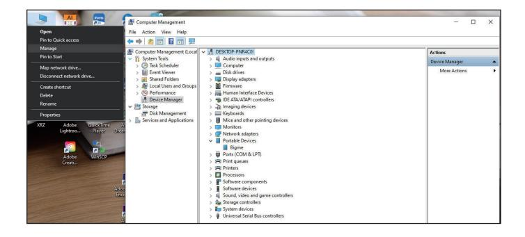
After the device is connected to the computer, right-click on the computer desktop [This PC], select [Manage] > [Device Manager] > [Portable Device-Bigme]
