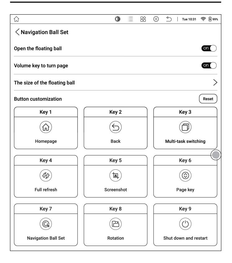
1. A control menu that floats on the top layer of the interface, you can customize the settings for 9 button functions
