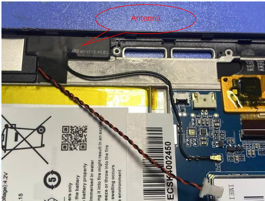
Photo 11 Internal of EUT
