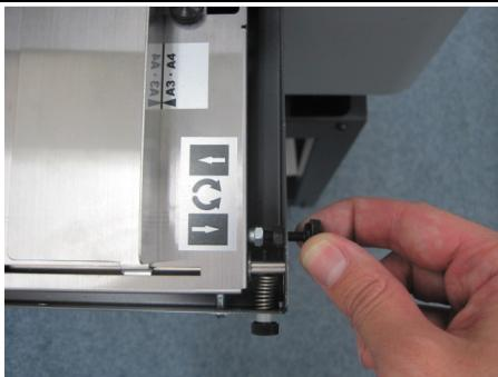
If necessary, adjust the position of the paper with the feed fine adjustment knob on the feeder tray.
