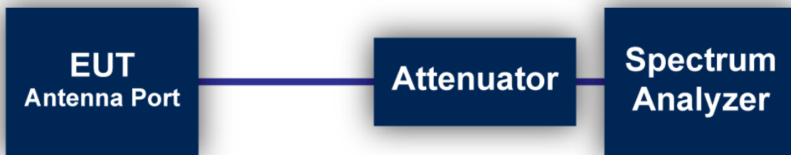
Figure 1: Direct Connection at the Antenna Port Test
