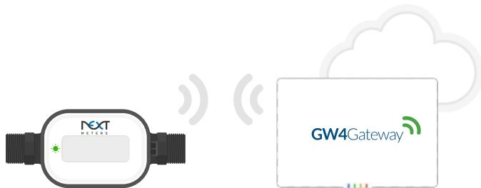
If green blinks are not seen, ensure the Gateway is online and any needed Repeaters are powered on.
