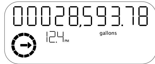
The LCD displays a meter read up to 10 digits, as well as the current flow rate and unit of measure. The flow indicator wheel spins when any flow is detected. The following status icons will show when applicable:
