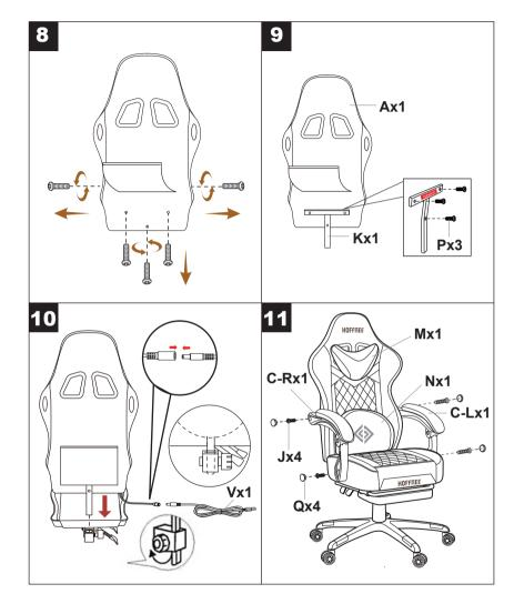
The four screws marked as "J" in the screw pack are an additional set of special anti loosening screws that can prevent the armrest from loosening, but the screws are not easy to unscrew after installation.
