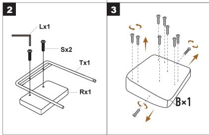
**Note:** All screws havebeenpreassembled to the accessories Please remove them from the accessories before assembling
