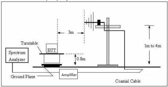
(C) Radiated Emission Test-Up Frequency Above 1GHz
