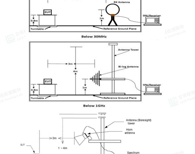
Above 18 GHz shall be extrapolated to the specified distance using an extrapolation factor of 20 dB/decade form 3m to 1m.
