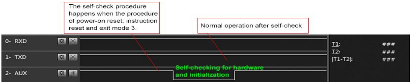
Timing Sequence Diagram of AUX when self-check
