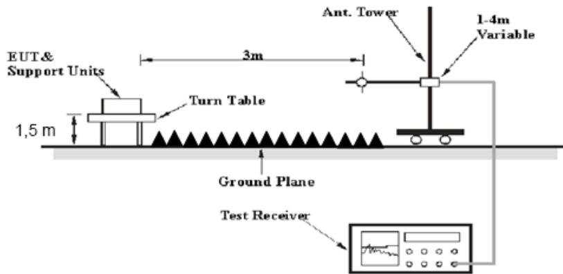
The radiated emission tests were performed in the 3 meters chamber test site, using the setup accordance with the ANSI C63.10-2020. The specification used was the FCC 15.209, and FCC 15.247 limits.
