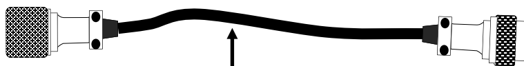
CONTROL ADAPTER FROM DONGLE CONNECTOR TO WELDER (TYPE VARIES BY BRAND, NOT NEEDED FOR SOME APPLICATIONS)
