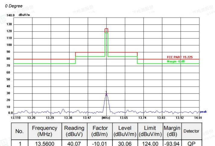
\*Note: Factor= Antenna Factor + Cable Loss
