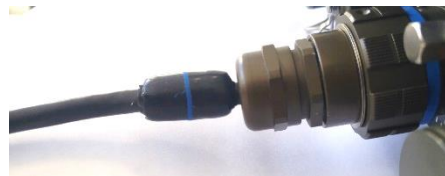
Figure 9: Self-Fusing Tape Application
