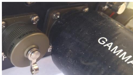
Figure 12: Collapsing Cold Shrink
