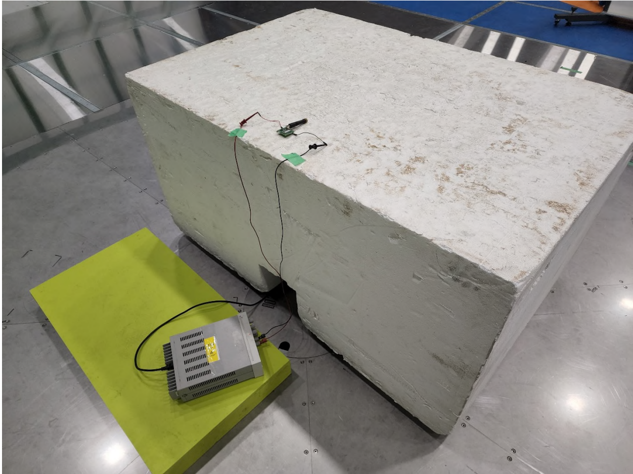
Figure 2 – Radiated Emissions Setup (Worst Case in X-Axis)
