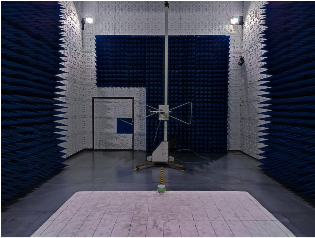
RADIATED EMISSION TEST SETUP ABOVE 1GHZ
