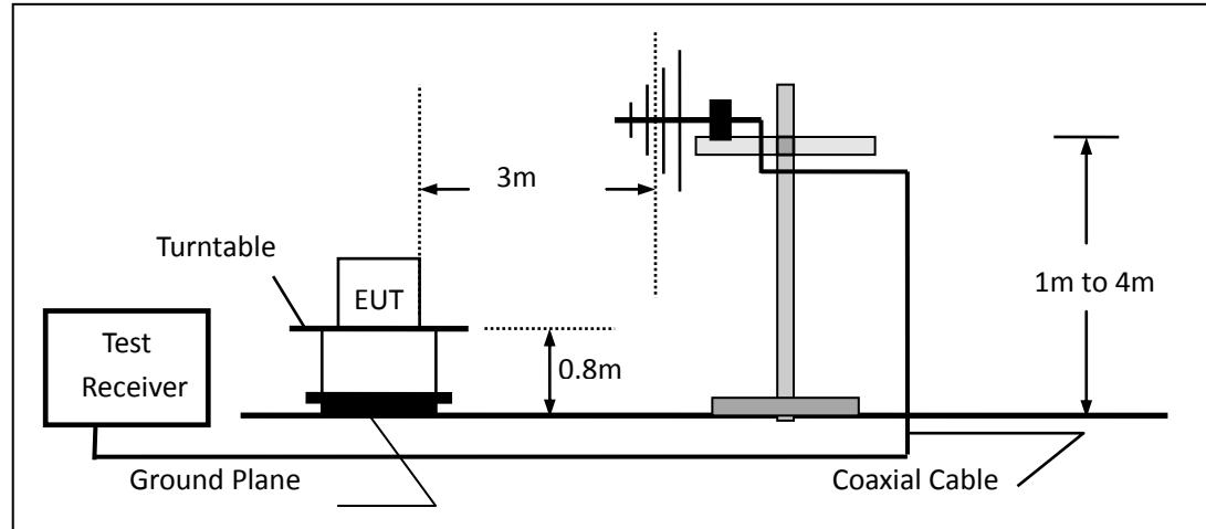
(c) For radiated emissions above 1000MHz
