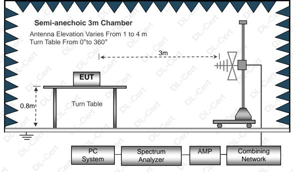
(C) Radiated Emission Test-Up Frequency Above 1GHz
