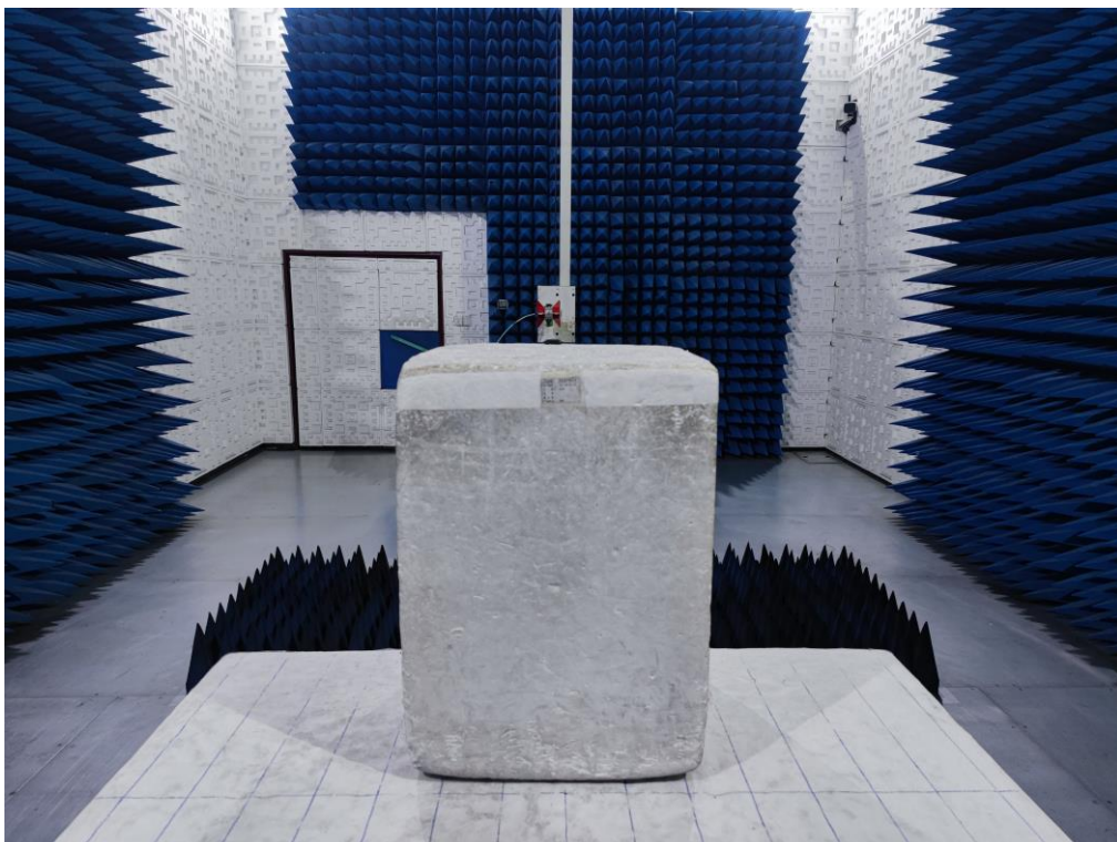
RADIATED EMISSION TEST SETUP ABOVE 1GHz
