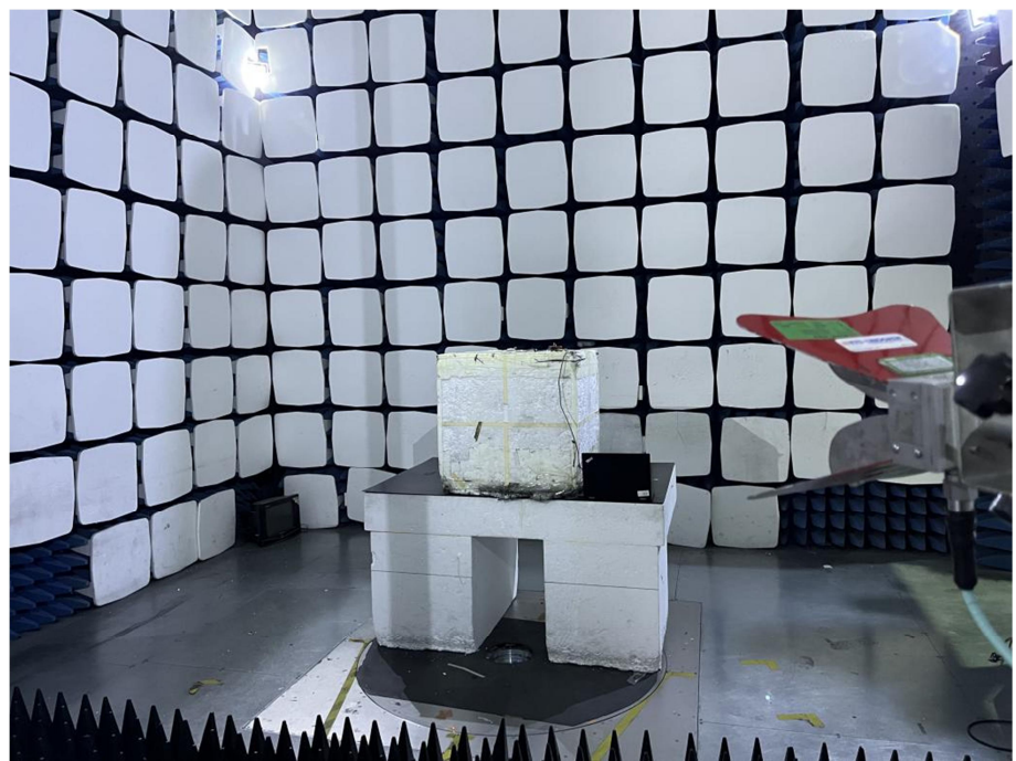
Radiation Emission Test Setup (1GHz to 18GHz)
