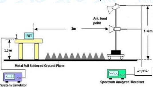
**Above 1GHz Test Setup**
