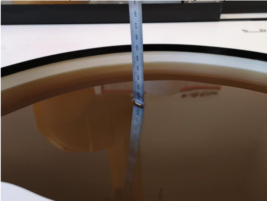
Photo 1: Liquid depth HBBL600-10000MHz Simulating Head Liquid
