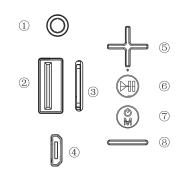
1.AUX: it can play audio via 3.5mm AUX cable to audio device
