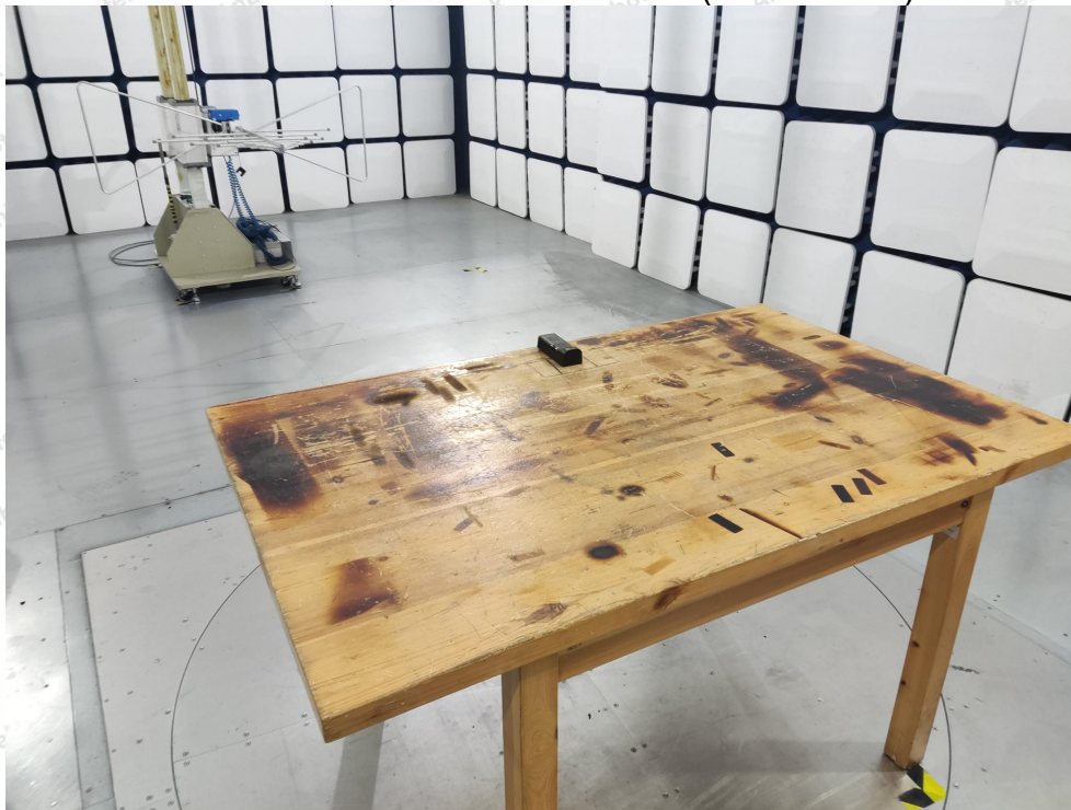
Photo of Radiation Emission Test (below 1GHz)
