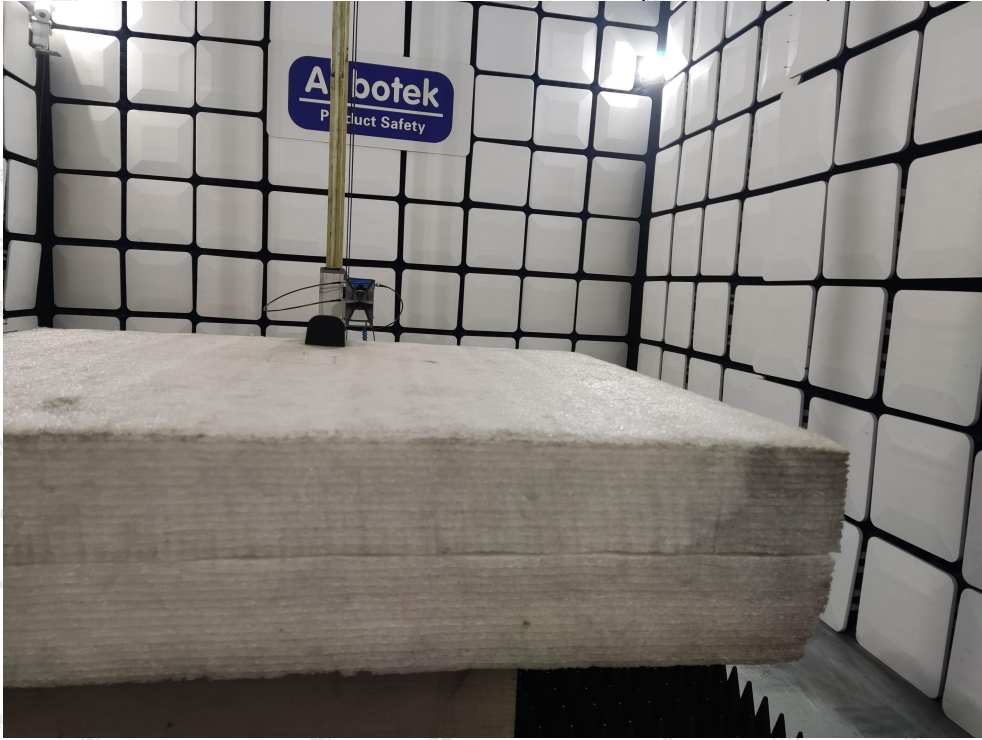
Photo of Radiation Emission Test (above 1GHz)
