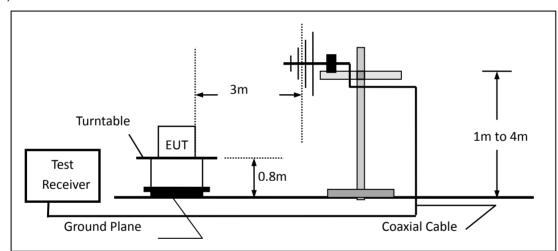
(c) For radiated emissions above 1000MHz
