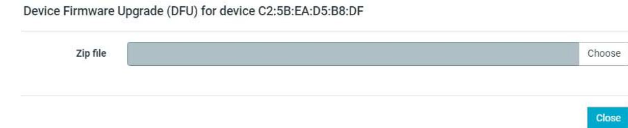
The DFU works with a single bank only. This means that if the firmware update is interrupted (power cut off or BLE disconnection), the application firmware will be corrupted, and the sensor will stay in DFU mode. The user will have to re-try the upgrading process. Note that the DFU MAC address is the sensor MAC address +1.
