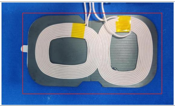
The antenna is Induction coil. The best case gain of the antenna is 0dBi.
