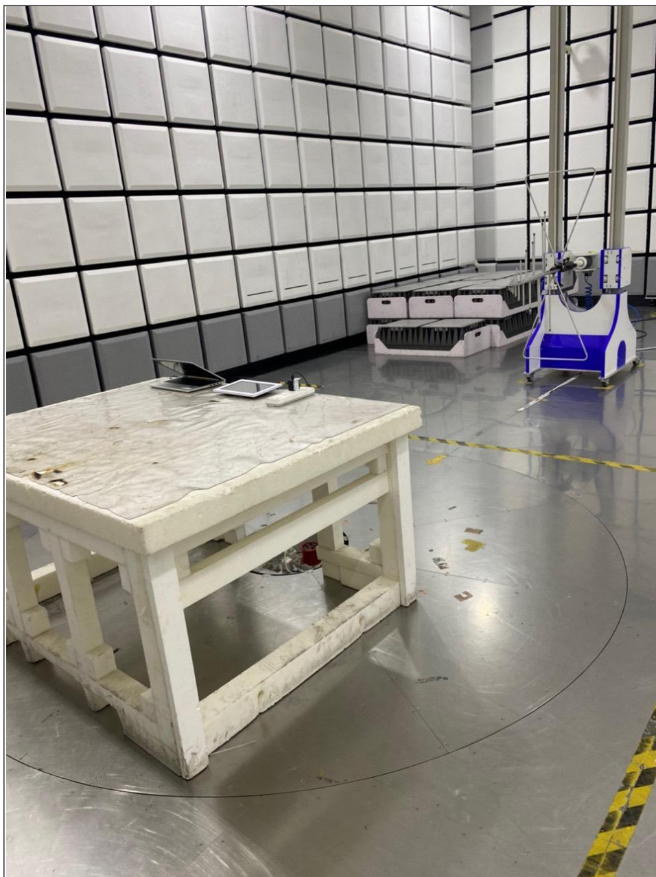
RADIATED EMISSION TEST (Below 1GHz)
