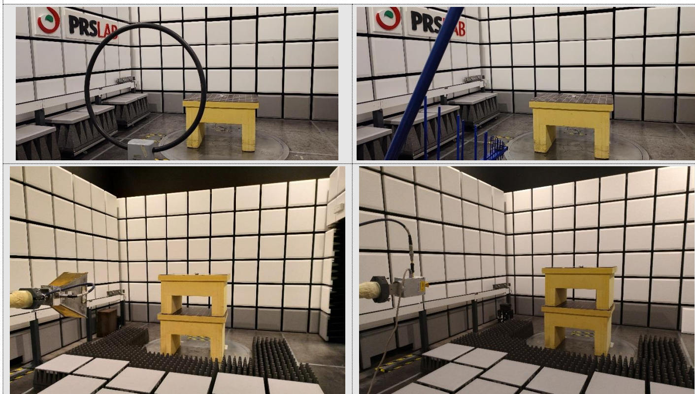
PHOTO N° 2 – RADIATED TEST SETUP
