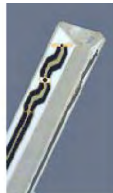
Figure 2.3 Probe Thick-Film Technique
