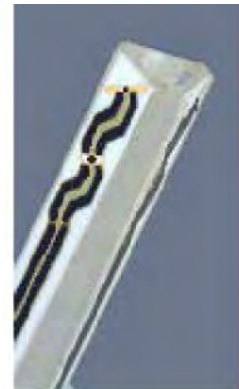
Figure 2.3 Probe Thick-Film Technique
