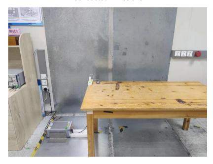
Radiated Emissions From 30MHz-1000MHz
